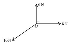
The diagram shows three coplanar forces acting at the point O. The magnitudes of the forces are  $6 \, \text{N}$ ,  $8 \, \text{N}$  and  $10 \, \text{N}$ . The angle between the  $6 \, \text{N}$  force and the  $8 \, \text{N}$  force is  $90^{\circ}$ . The forces are in equilibrium. Find the other angles between the forces.
