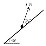
A particle of mass  $0.12 \,\mathrm{kg}$  is placed on a plane which is inclined at an angle of  $40^\circ$  to the horizontal. The particle is kept in equilibrium by a force of magnitude  $P\,\mathrm{N}$  acting up the plane at an angle of  $30^\circ$  above a line of greatest slope, as shown in the diagram. The coefficient of friction between the particle and the plane is 0.32. Find the set of possible values of P.
