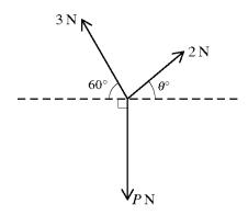
The three coplanar forces shown in the diagram have magnitudes 3 N, 2 N and P N. Given that the three forces are in equilibrium, find the values of  $\theta$  and P.
