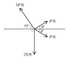
The four coplanar forces shown in the diagram are in equilibrium. Find the values of P and  $\theta$ . [5]
